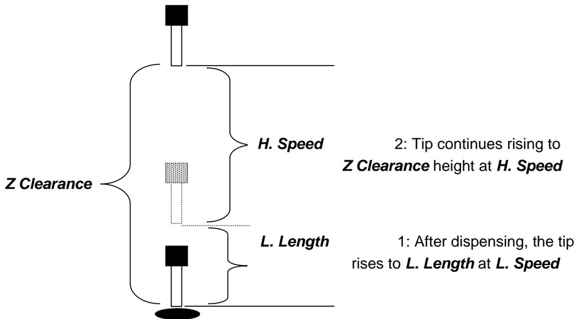
Values for **H. Speed**, **L. Speed** and **L. Length** are registered with the **Dispense End Setup** function by pressing the **F4** key, then choosing **Dispense End Setup**.
