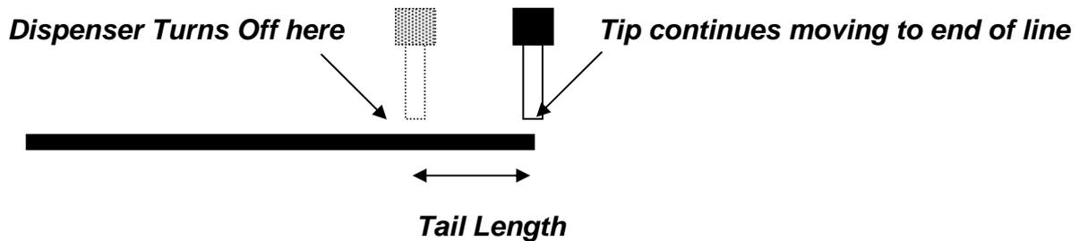
Values for the *Head Time* and *Tail Time* used when performing line dispensing are registered by pressing the **F4** key, then selecting **Line Dispense Setup**. The set values will be used by all lines from that memory address forward until new set of *Line Dispense Setup* values are found.
