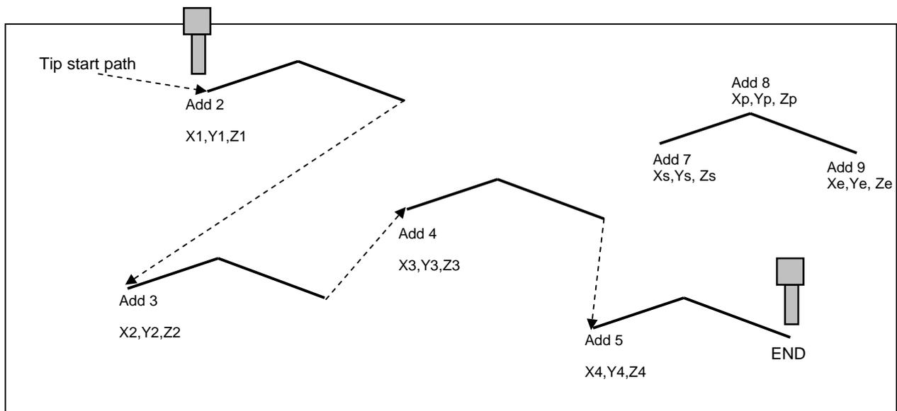
Addresses 7, 8 and 9 comprise the subroutine that will be executed whenever it is called within the main program. The coordinates in the body of the subroutine (Xs,Ys,Zs, Xp,Yp,Zp Xe,Ye,Ze) are not important; *the critical information is the relative position to each other*. The actual work will be performed on the coordinates in the main body of the program.
