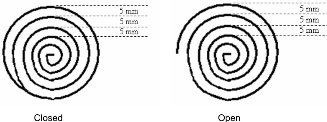
An open or closed option is also available for this function. Selecting the Closed option will make a whole circle first before making the spiral. Selecting the Open option will make the spiral without closing the outer circle.
