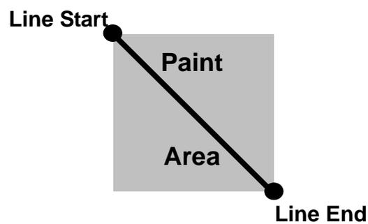
If, for example, a brush width of 5 mm was used, the tip will take the following path when the program is run:
