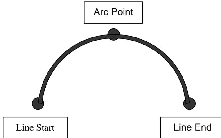
Lines and arcs can also be combined to dispense a bead of material along a complex path:
